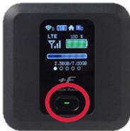
Keep holding the power button until "FUJISOFT" is displayed on the screen.
